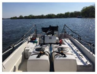
Our staff has access to five fully equipped application vessels with eight fulltime and two seasonal licensed applicators. The application will utilize our customized 18-foot Carolina Skiff boat equipped with a two-tank, sub-surface injection system. Each product tank is operated using a dedicated calibrated rate controller through an assigned set of hoses, allowing us to apply up to two different non-compatible active ingredients at the same time.
